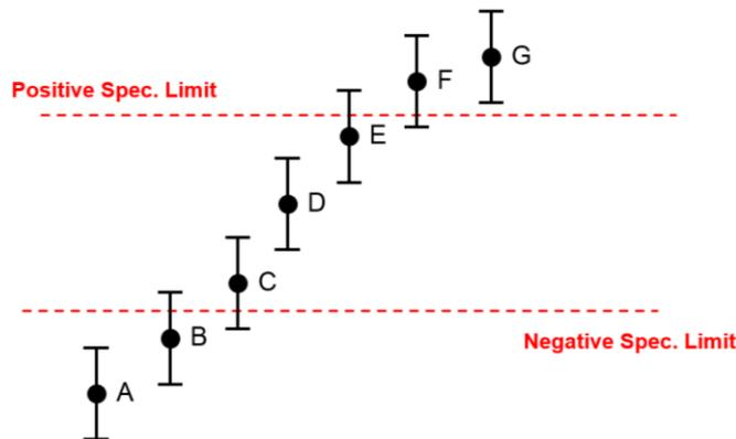
In this illustration, only measurement D would meet the specifications. Measurements A and G are the only measurements which are definitely beyond the specification, but all others may either be in, or out of specification.
