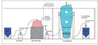
Wet granulation with high-shear mixer granulator and dryer
