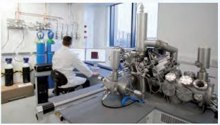
Time of flight secondary ion molecular spectroscopy instrument used for surface analysis
