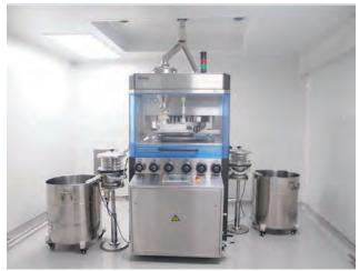
Tablet compressing set, granule transfer tube, tablet deduster and bulk product IBC
