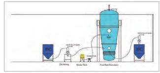
Wet granulation with fluid-bed granulator
