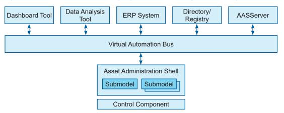
Figure 2.4: Overview of the Eclipse BaSyx System Structure (Adapted from "BaSyx Overview" [12])
