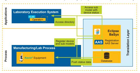
Figure 3.5: Architecture of the AAS in Eclipse BaSyx (Adapted from "Eclipse Wiki – BaSyx Overview" [13])
