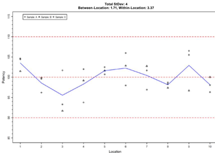
micromixing), high between-location variance (hot and cold spots in the blend—poor macromixing), and both high within-location and between-location variance (incomplete mixing).
