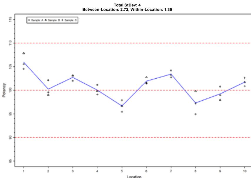
Figure 4: Plot showing both high within-location and high between-location variances (incomplete mixing).
