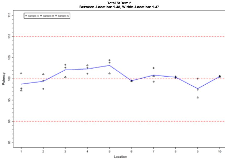
Figure 2: Plot showing high within-location variance (poor mixing on a unit dose scale—poor micromixing).
