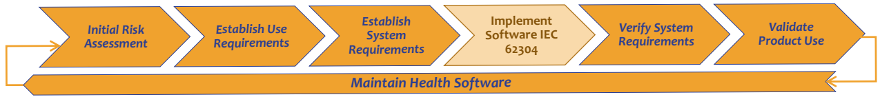
Figure 4: Health software product life cycle based on IEC 82304.
